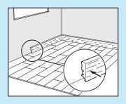
When the new flooring meets a treshold or a doorway, we recommend undercutting the moldings. To secure the right cut, turn a plank upside down and place it on the floor up to the door frame. Then place a hand saw flat against the plank and simply cut through the door frame. Remove the cut out and vacuum away debris.
