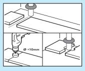
In case of a double pipe, drill a hole at each of the marked points that is equivalent to the diameter of the pipes.
