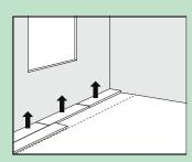
Apply the vinyl glue on the floor for about the same width as the two first rows. Always take into account the instructions of the vinyl glue. We recommend to use the specifically developed branded vinyl glue.
