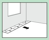
Use a heavy roll to ensure the best bonding and adhesive transfer. Wait no longer than 30 minutes before rolling on the installed area.
