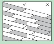
Measure the room before you start fitting. Make sure that the last row of panels is at least 5 cm wide when finishing the installation.
