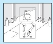
If located on the long side of the plank, make a 45 degree cut from each hole to the edge of the plank. Then glue the piece in place. Fill the joints around the pipe.
