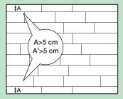
We recommend to dry fit first (without glue). Start the first row with a whole plank in lenght.
